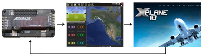
Fig. 2 Hardware-In-the-Loop (HIL) simulation feedback loop
