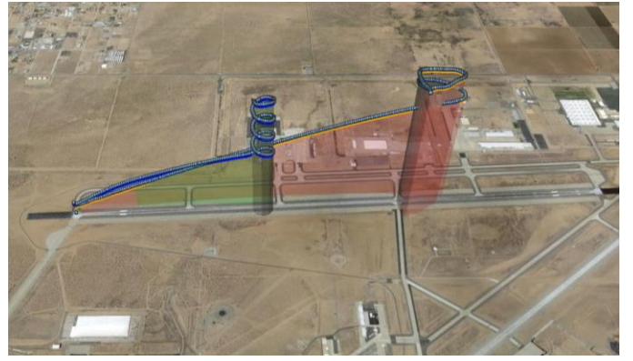
Fig. 5 The flight paths of plane one (red) and plane two (green) when plane one has three way points.
